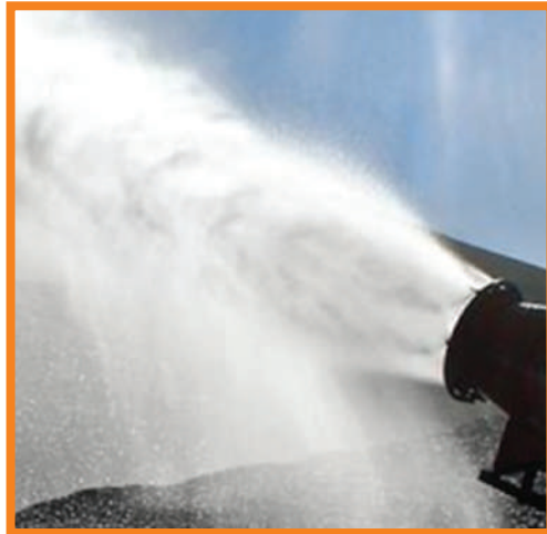
Figure 22: Water cannon to suppress dust emissions
